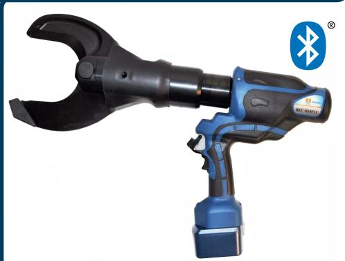
The **REC-B105YC** is designed to cut copper and aluminum cables as well as lead-sheathed telecommunication cables. The extremely large jaws and scissortype blades allow for easy cutting of large underground cables. The sidebar handle allows the user to stabilize and balance the tool.
